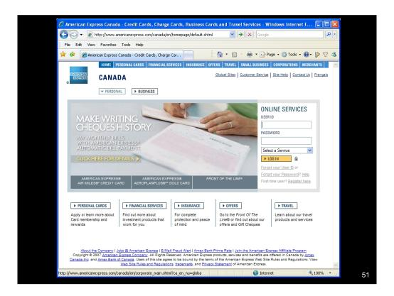
Here the AMEX page is asking for the User ID and password, but there is no SSL connection so there is no indication that the transmission would be sure, other than a loc icon right on the page.
